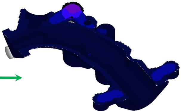
Solidification time analysis shows better solidification results and the last solidifying region is inside the feeder and casting will solidify before the feeder. So it is resulted in shrinkage free casting.
