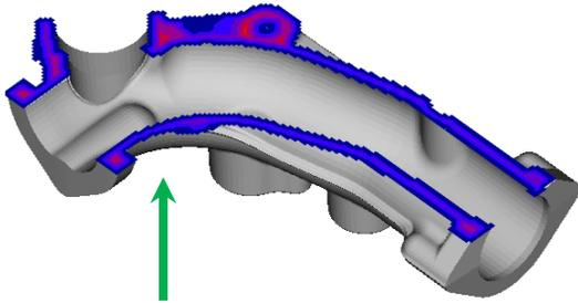
There are several thick regions in the casting at boss sections. Thickness analysis shows mass concentration in the bottom portion, corresponding to an inscribed sphere diameter of 33 mm.
