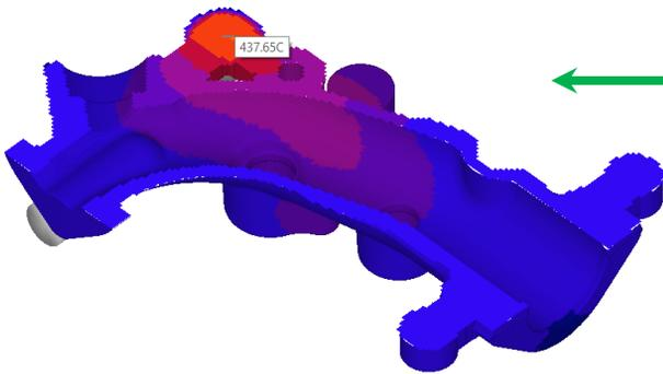
Solidification temperature analysis shows isolated temperature region inside the feeder. So casting is free from shrinkage defect.
