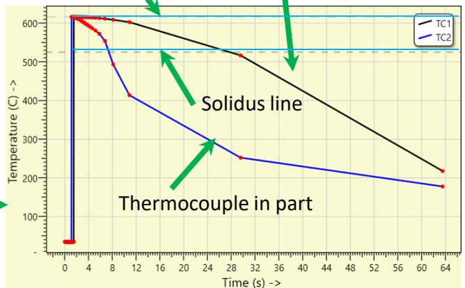
Thermocouple analysis reveals that thermocouple in part region crosses solidus temperature earlier and thermocouple at feeder crosses solidus afterwards thus feeder solidifies last.
