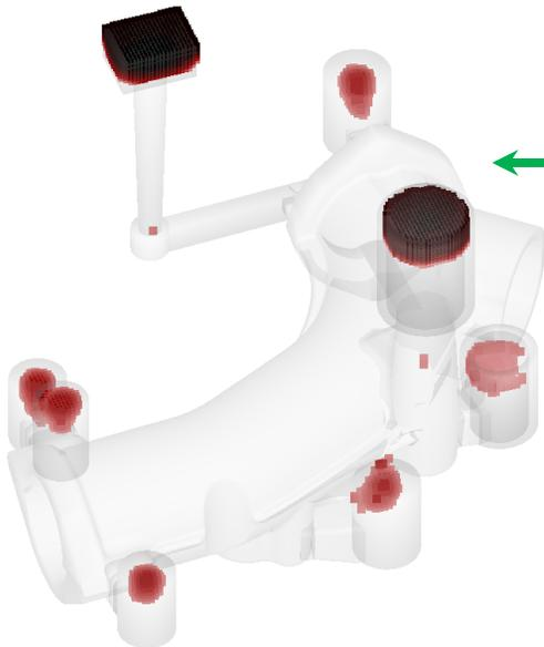
Shrinkage porosity results also shows that it is observed in the feeders only. Shrinkage porosity from casting is completely eliminated.
