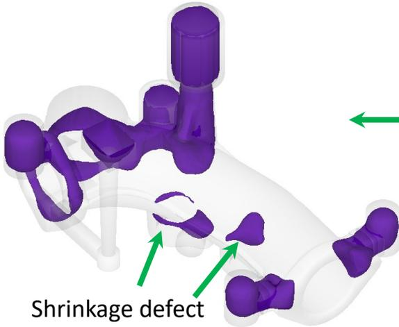
Liquid fraction shows metal solidifying last in the thick ring section of the casting which leads to porosity . Two isolations are observed at bosses in bottom portion of the casting.
