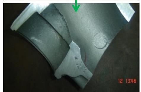
The current methoding of the casting included two top feeders and three side feeders connected at bosses. Also three chills are placed at bottom thick sections.
